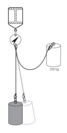
The 200 kg test mass is secured with a force measuring device to the anchor point.
