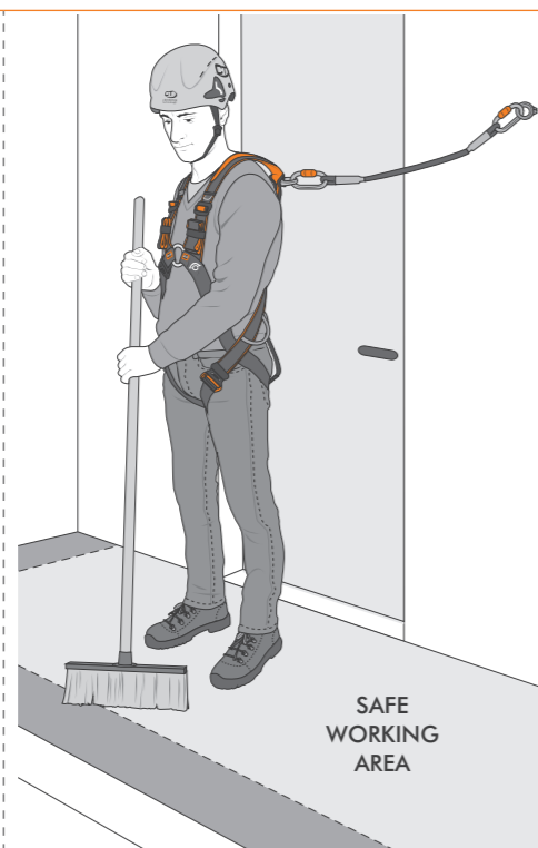
11.2 - Working on a horizontal surface
