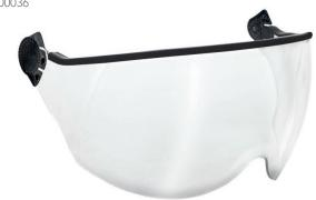
Polycarbonate visor with scratch-resistant coating and anti-fog treatment. The rubber profile on the upper edge protects in case of dripping and the cut proof edge ensures maximum comfort. The ergonomic and panoramic shape is compatible for overlapping corrective glasses. Screw set for mounting is included with visor.
